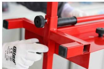
6. Slide the all the 'red holders' against the box. Tighten the black knobs to fix the box.
