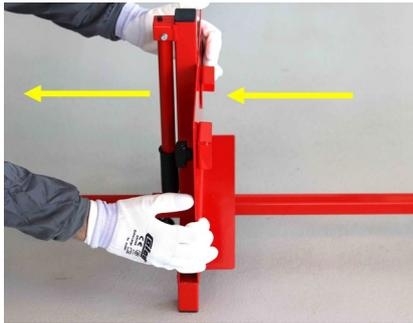
3. Loosen the black knobs at the bottom, at the wheels. Slide the 'red holders' out as far as possible. Tighten the black knobs so that the 'red holders' remain upright.
