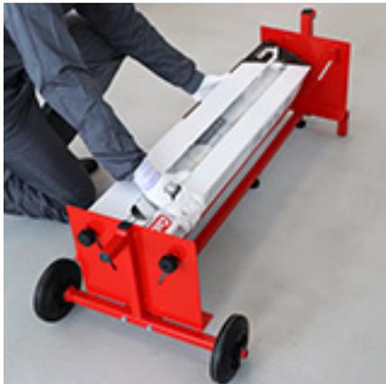
5. Slide the top (with the handle) against the box. Tighten the black knobs from the top to the central rod to fixate the top part.
