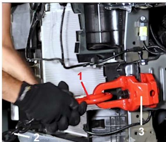
FIGURE 4.16 – CHAIN (2) HOOKED (1) TO A CLAMP (3) OR DIRECTLY TO THE POINT ON THE VEHICLE TO BE STRAIGHTENED
