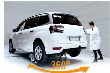
Wheel used to rotate the vehicle up to 360°.
