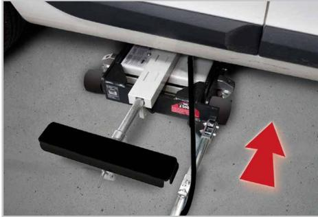
Its design makes it easy to slide it underneath the vehicle (14 cm in low position).
